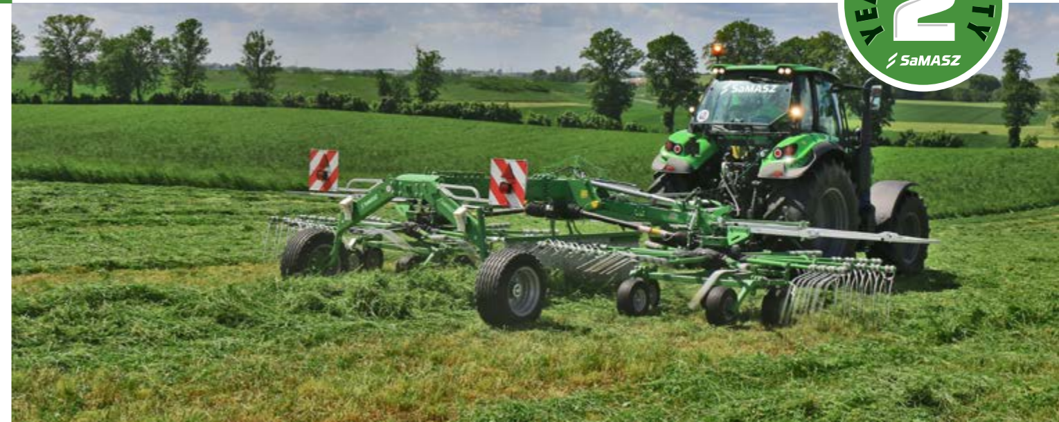
Fig. A. Variable working width within 7.20 and 7.60 m (23'7"-25'), Z2-840 (7,60 - 8,40 / 25' - 27'7") range. Adjustment is possible only in transport position by inserting a pin.
